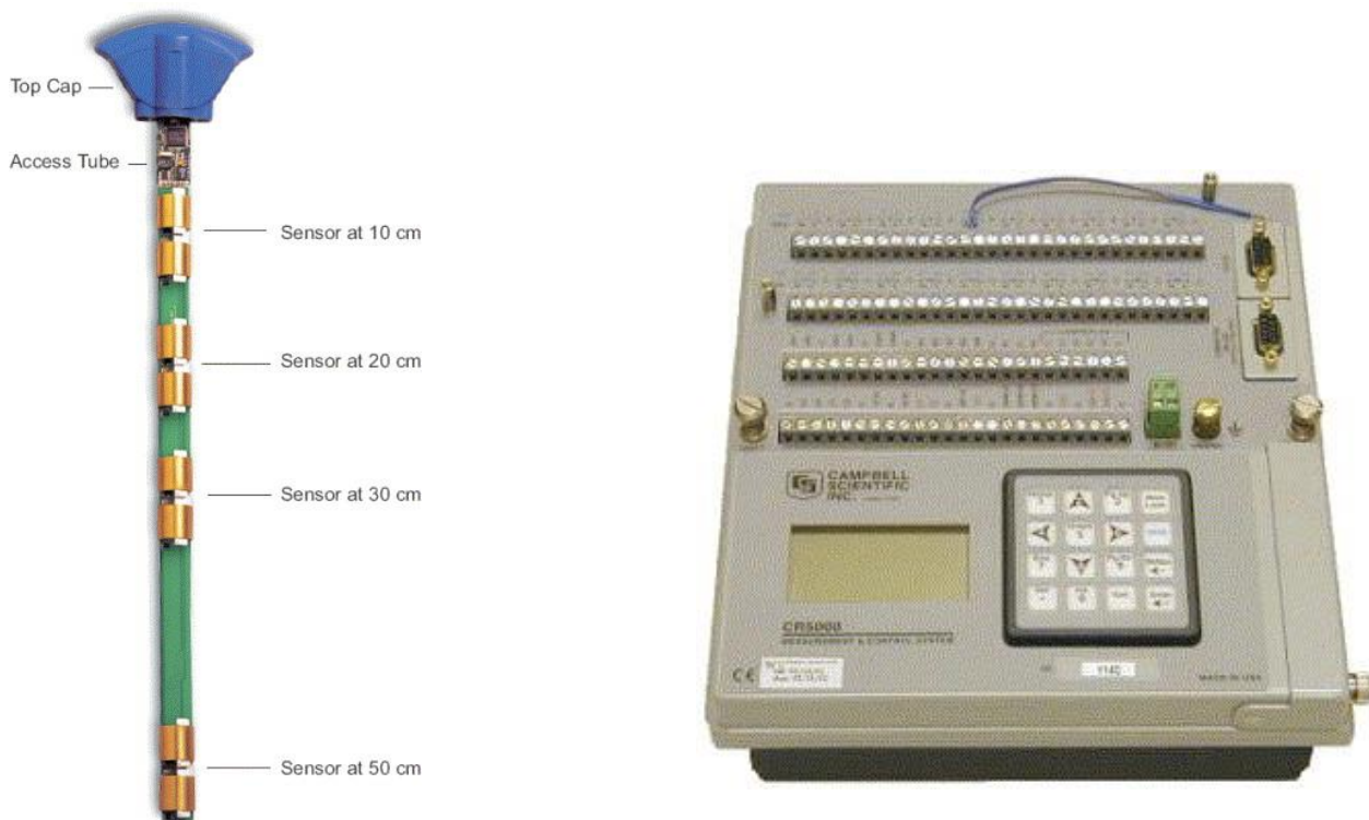
Fig.2. Wireless Underground Sensors and Data Acquisition Devices
