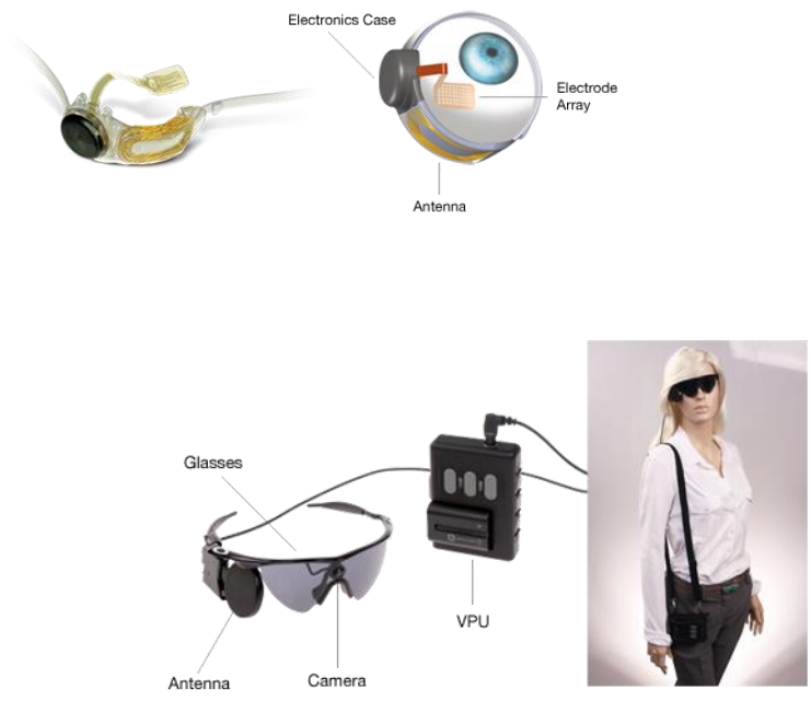
Fig.2. The structure of Argus II. [8]
