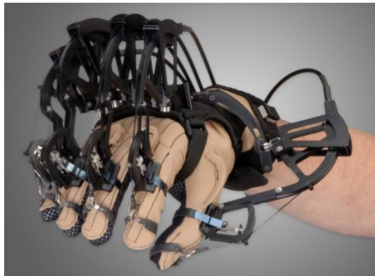
Fig.9. CyberGrasp; Courtesy of CyberGlove Systems LLC, California
