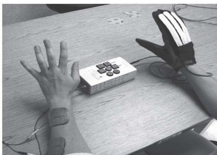
Fig.2. Contralaterally controlled functional electrical stimulation
