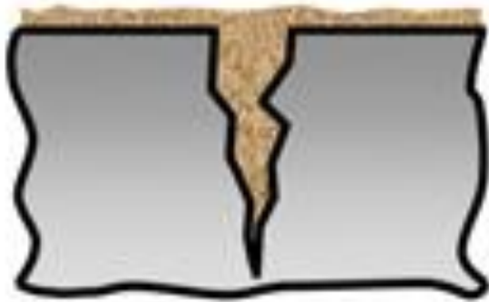
1 Crack filled with dirt
