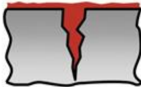
3 Application of penetrant
