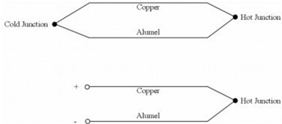
If this circuit is broken at the center, the net open circuit voltage (the Seebeck voltage) is a function of the junction temperature and the composition of the two metals.
